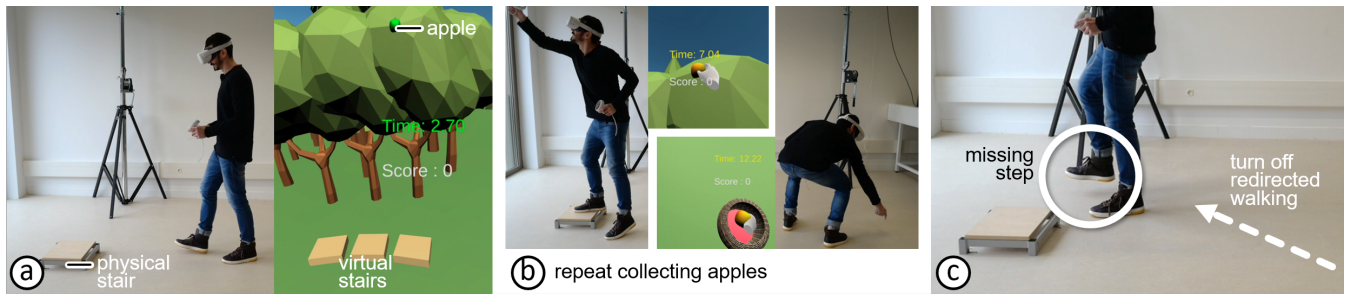
Figure 1: (a) The SteppingOn setup has one physical and three virtual stairs. (b) We redirect the user to match the stepping feedback when the user is walking back and forth and collecting apples on the stairs. (c) The application randomly turns off redirection to create a missing step.
